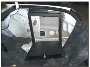
Position frame assembly as shown. Trunk liner does not have to be removed, but you may want to cut it as needed to improve access for routing wires.
